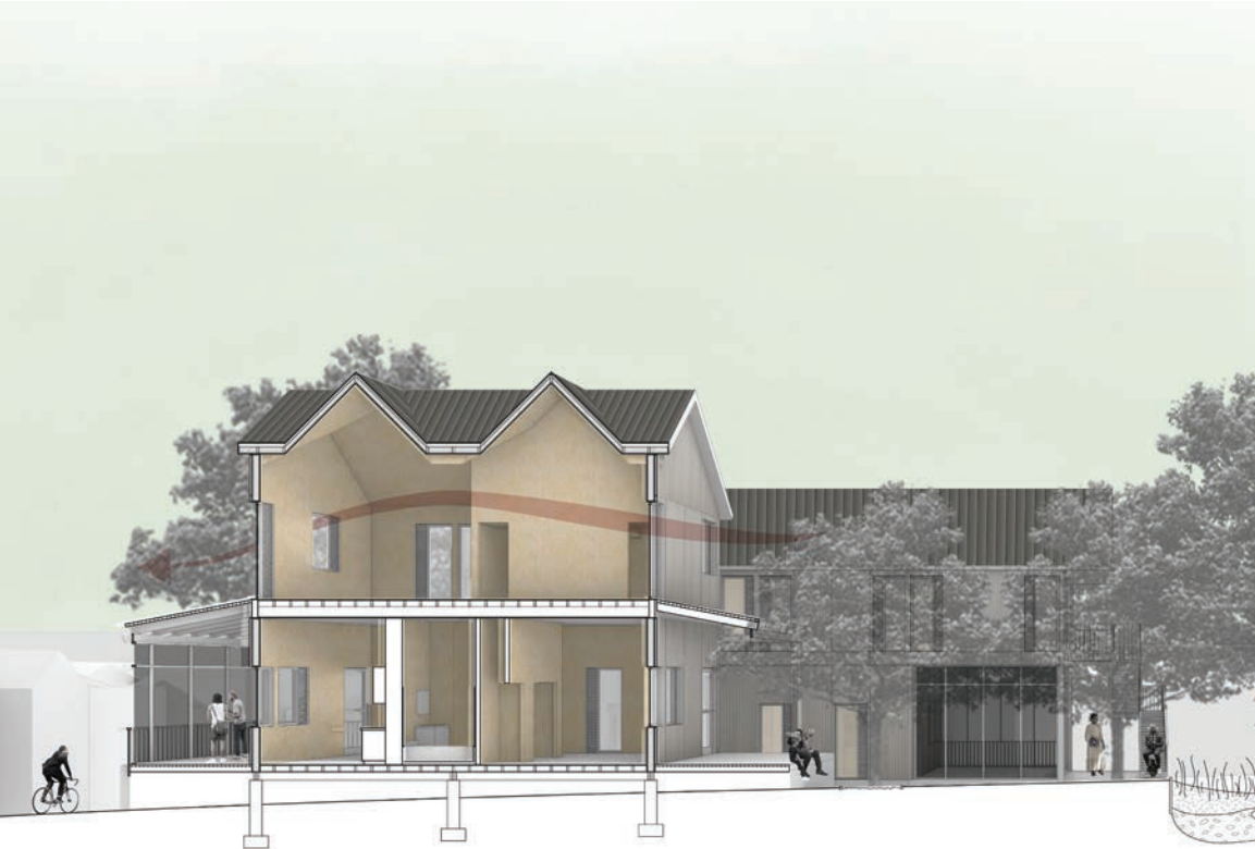
Cross section of the project highlighting the the spatial design allowing cross ventilation on both floors.
